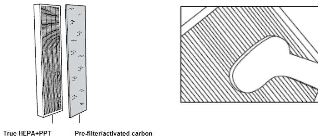
**Signs for used up filters:** increased sound, reduced air flow, congested filters, rising presence of smells. The filter needs to be replaced by a new one when the **HEPA filter** changes its color from white to grey or black. If the HEPA filter remains white, there is NO need to replace the filter.
