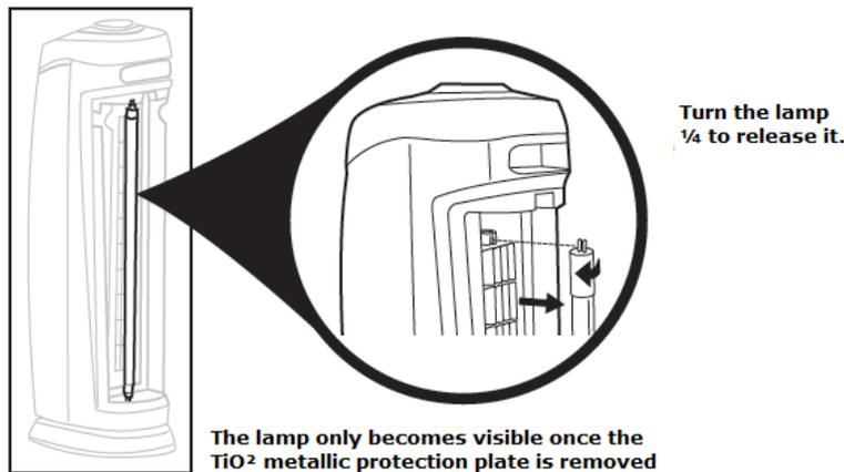
9. Reposition the UV-C lamp horizontally by inserting the pins (top and bottom) into the slots and turn the lamp 1/4<sup>th</sup> of a turn to snap it.
